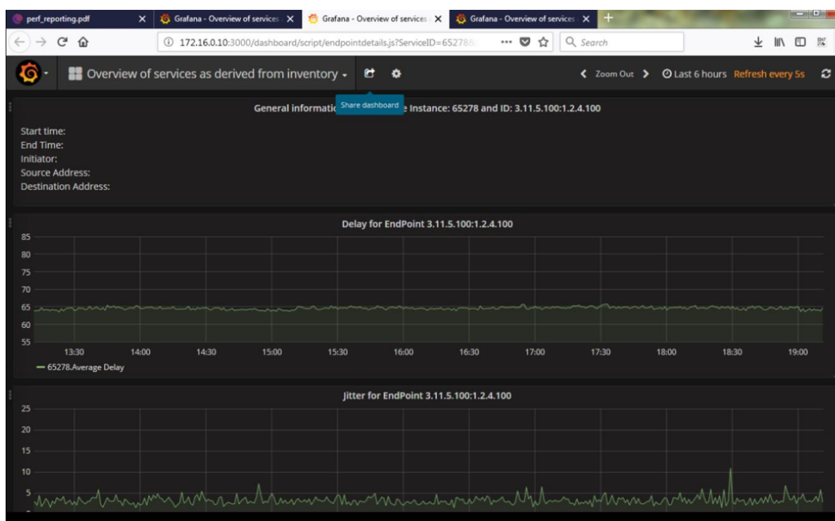
Figure 6.4: Example of delay and jitter test screens for service 65278 between MA2 and MA3 devices
